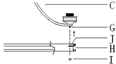
5. By measuring determine correct number of links needed for proper hanging height. Use a pair of pliers to open one link of the Chain (C2) then remove the excess Chain (C2) and discard it.
