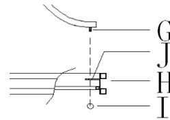
5. By measuring determine correct number of links needed for proper hanging height. Use a pair of pliers to open one link of the Chain (C2) then remove the excess Chain (C2) and discard it.
